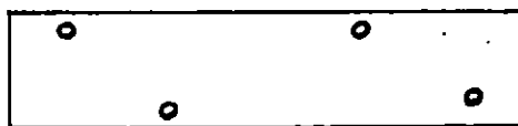
Sl. — Fig. 4. Jedan od načina mjerenja debljine piljenice — One of methods of measuring the thickness of the board
